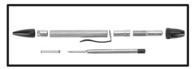
The Atlas is shorter and requires a spacer on the mandrel or the use of an adjustable length mandrel. Tip projection is adjusted by pressing retainer into the TOP portion of the tube and checking with the refill.
