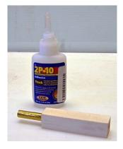
I sand the ends of my pen blanks using a disc Sander and a 90° fence. The end is well sanded when the shiny brass tube is revealed uniformly at each end.
