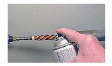
Three top coats of spray Krylon give me the right high-gloss finish and protection for the pen. After an additional 24-hour drying, the pen blank may be buffed and or waxed if you desire.
