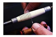
In order to mark out longitudinal lines it is necessary to have an indexing system on your lathe. Most modern mini lathes have 12-24 division indexing built-in. My older Powermatic lathe does not have indexing so an external commercial plate was purchased and used.
