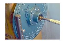
To burn these horizontal lines I use a commercial pyrographic instrument; mine was very inexpensive. I have mounted the pen between two blocks of wood to allow it to lay flat on a support table attached to my lathe's banjo.
