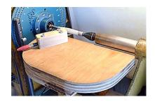
The lines are burned by lightly dragging the pen along the table from one end of the blank to the other.
