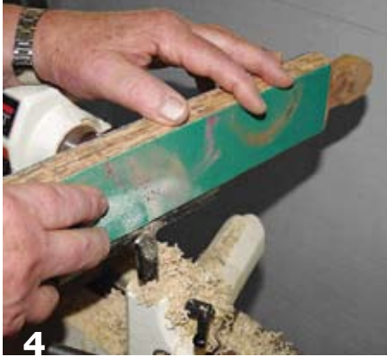
4 With the lathe running at a slow speed, flatten the glue block with a sanding stick.
