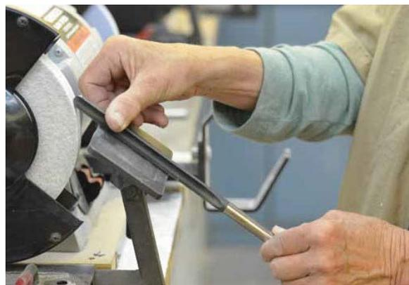
10. Sharpen a conventional gouge by rotating it against the wheel.
