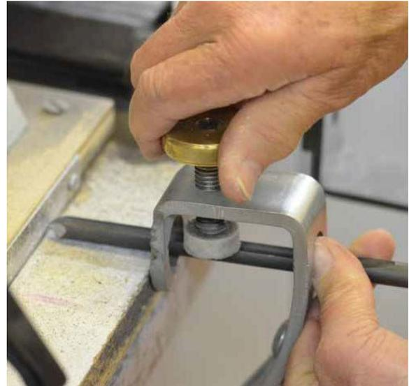
11. With the stabilized gouge fixture set the tool projection length.
