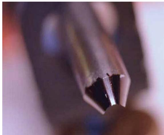
4. The fixture is properly adjusted to the tool bevel.
