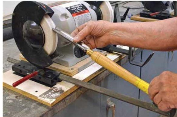
5. To sharpen the SRG in a long arm fixture use a light downward pressure.
