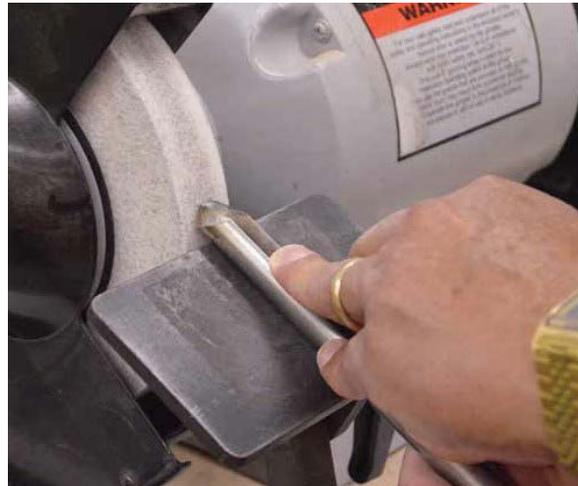
13. Adjust the platform to match the gouge bevel angle.
