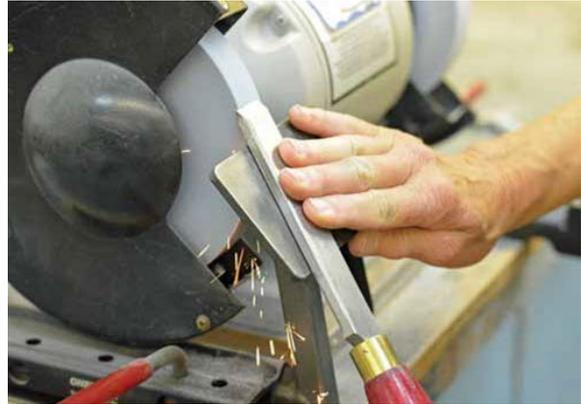
8. Hand sharpening a skew chisel with a matching angle platform is safer.
