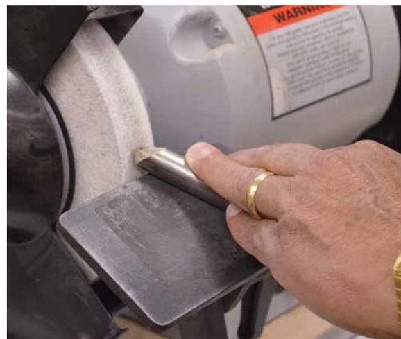
14. Start the sharpening by rotating the tool and sweeping it to the right.
