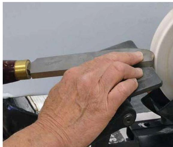
17. Sharpen scraper by laying it flat on the platform and rotating it against the course wheel.
