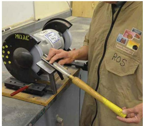
6. A safer method is to hand sharpen the SRG
