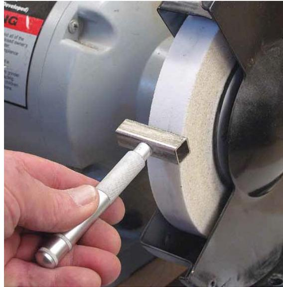
1 . An inexpensive diamond wheel dresser is necessary to keep the wheels clean.
