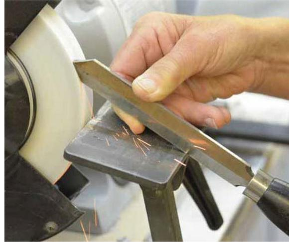
18. Parting tools start with the heel of the bevel against the wheel, then the handle is raised.
