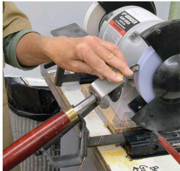
12. After setting the arm length, sharpen one side by rotating the tool to the right, then the left side.
