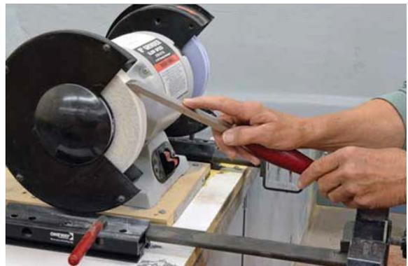
7. Set the right face of the skew chisel using a “T” fixture & set the opposite face on the opposite side of the “T”..
