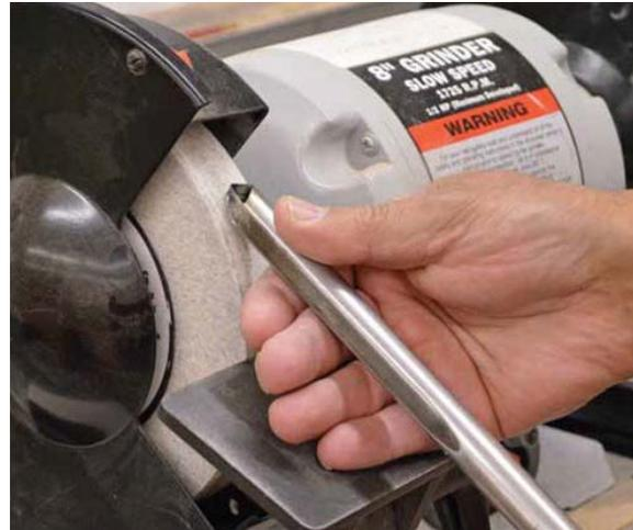
16. Free hand sharpening can also be done by pushing the tool upward while rotation.
