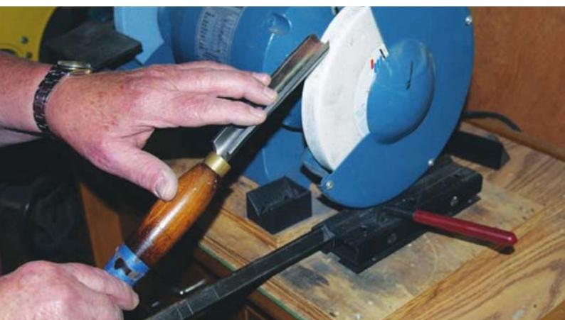
Better: Create a more acute bevel angle on your tool, which will place it higher up on the wheel in a safer position when sharpening.
