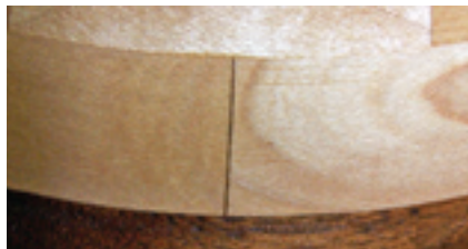
Error in cutting the segment angle accurately
