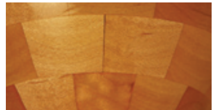
Tenting caused by glue squeeze-out on back side
