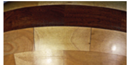
Multiple errors in segment angle cutting
