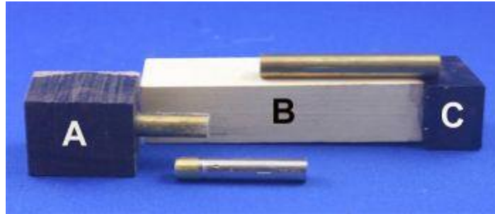
Figure 4: The blank sections cut, drilled and ready for the tubes to be glued in place.
