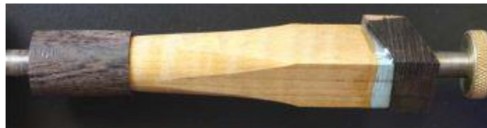
Figure 7: The blanks arranged and mounted on the mandrel for turning.
