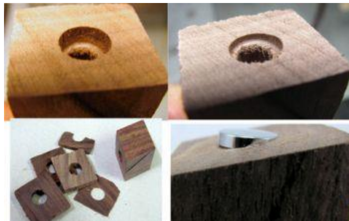
Figure 5: Section C with both holes sizes drilled.
