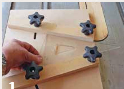
1 Use a 30/60/90 triangle to set the fences on your table saw sled to the desired angle.
