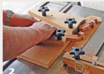
2 Cut the individual segments. The length of all segments is made identical with the use of an adjustable stop (bottom right of photo).
