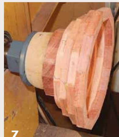
7 A completed bowl blank built from four segment rings and a solid layer for the bowl's foot.
