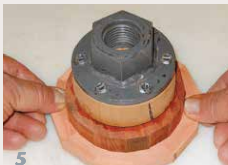
Three methods of centering a ring when gluing it to the previous layer. Use a ruler or your fingers as a gauge, or mount the ring in large chuck jaws mounted on your tailstock.
