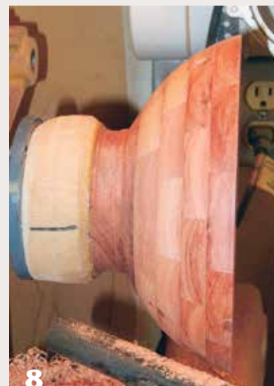
8 The outside profile turned. Leave the foot material thick for added stability during turning near the rim.
