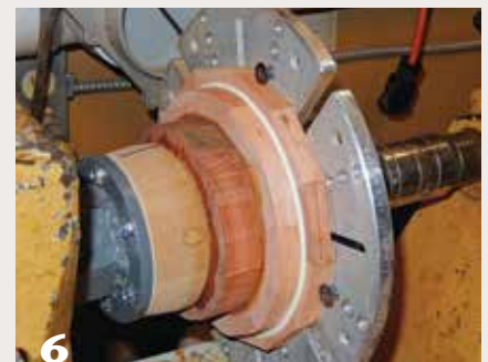
Three methods of centering a ring when gluing it to the previous layer. Use a ruler or your fingers as a gauge, or mount the ring in large chuck jaws mounted on your tailstock.
