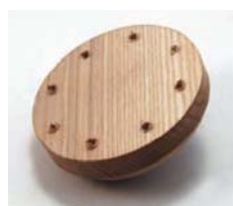
Glueblock with holes not pre-drilled. Mushrooming of the wood will prevent getting a good glue joint.
