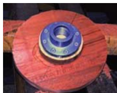
Faceplate, glueblock, and platter, assembled and ready to turn.
