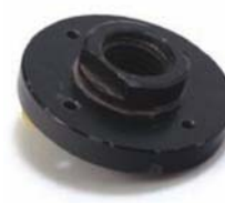
Glueblock with holes not pre-drilled. Mushrooming of the wood will prevent getting a good glue joint.
