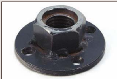
Locally made faceplate with threads relieved.
