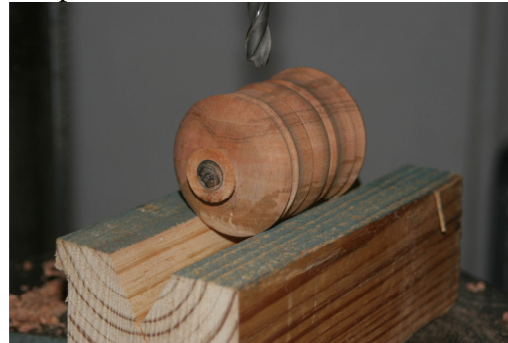
vee block assist the drilling
