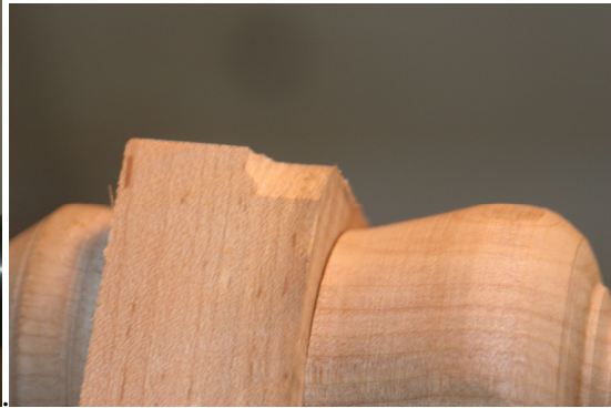
Roughing the face grain blank
