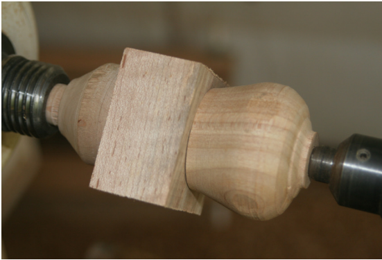
Blank on Morse taper Mandrel
